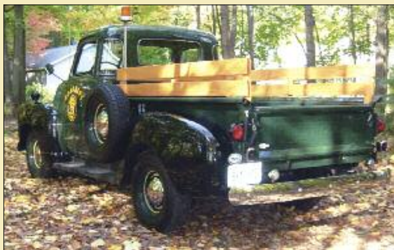
The side-mounted spare tire and the orange service light were added during the restoration. The recently-added back-up lights and passenger side tail light are correct "Guide" accessories.
