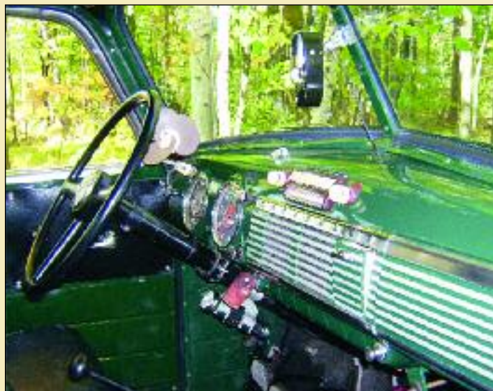
Notice the rubber-bladed Casco electric fan which was added to the dashboard using the same attaching holes that were there before the truck was restored.
