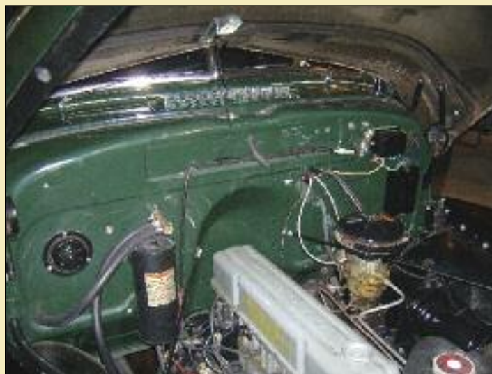
The engine is out of a 1955 Chevrolet. Notice the radiator overflow tank on the firewall and the rare under-hood lamp.
