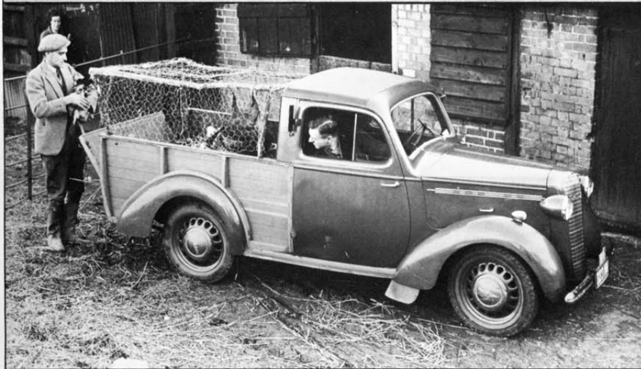
Based on the H-type Vauxhall saloon, the HC 5/6 cwt van (top picture) appeared early in 1938 and was claimed to give 35 mpg fully laden. The 6 cwt Utility Wagon (above) based on the HC was launched in 1939. The larger, 10/12 cwt JC van looked almost exactly like the HC. Two pictures below show some of the main changes made to the W models in mid-1938. Behind the more modern radiator grille sat a more powerful, 72 bhp engine. The radiator filler cap was now out of sight under the bonnet. The 30 cwt WS still sported its original disc wheels; lower picture shows a 3-ton short tipper complete with A.R.P. equipment. Note the difference in bonnet lengths between the 30 cwt and 3-ton models.
