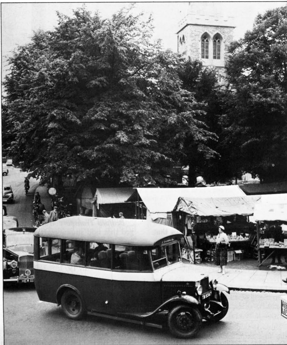
In August 1931 came modified versions of the 2-ton chassis for bus bodywork, the WHB for 14-seater bodies, the WLB for 20-seaters. The Waveney-bodied 14-seater (above) was the very first bus to be built on this chassis; it has now been faithfully restored by Bedford dealers Arlington Motors. The Plymouth owner of the Duple-bodied 20-seater (below) called the Bedford "far and away the best 20-seater on the market".
