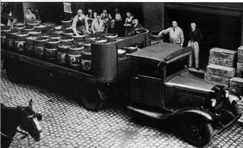
Six-wheeler conversions (above) and articulated outfits appeared during Bedford's very first year. Both Baico and Spurling soon offered chassis extensions and third axles. Oddly, the very early 2-tonner at left above sported single rear wheels, unlike the more usual twin
