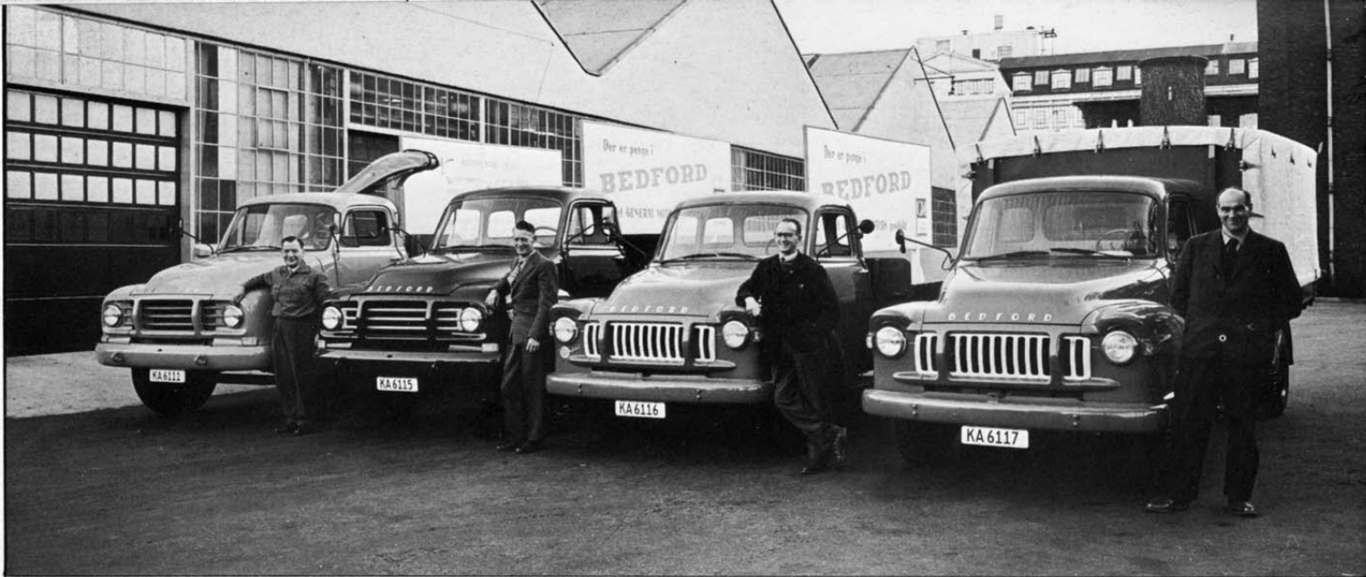
The new look in normal-control Bedfords, first seen at the 1958 show. Picture above shows the two TJ cab versions – vertical grille slats and headlamp ‘eyebrows’ up to the 4-tonners, horizontal slats for the heavier jobs (on the left in the picture above, taken in Denmark). Top picture, facing page, shows four generations of bonneted Bedfords
