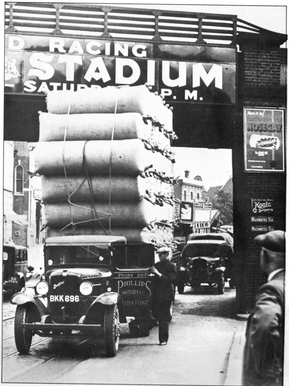
The owner of the 2-tonner above seems to have taken very literally the 1933/34 Bedford claim as "the truck for a 50% overload". The vehicle is actually a Carrimore artic outfit based on the 2-ton short chassis, with a load of hops from Kent to London. Below, short- and long-wheelbase 2-tonners; the vehicle on the left is a very early Bedford, registered before the end of 1931. The Express Dairy vans feature a very deep windscreen and, apparently, sliding door windows.
