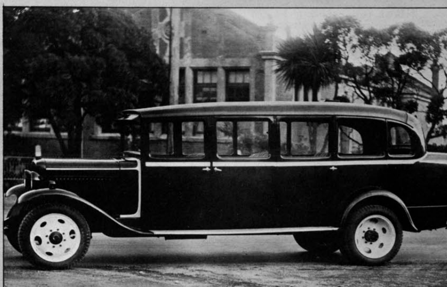
right was built in New Zealand on an early WL2 2-ton chassis. When is a truck not a bus not a car? When it's all three in one, presumably! The days of these odd vehicles seem to have gone now.
