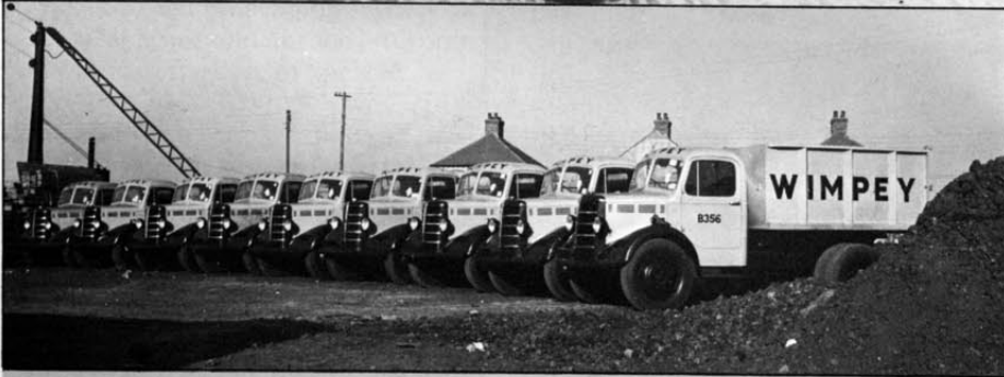
The OS and OL 5-tonners made a great name for themselves. The long-wheelbase (157 in.) model in the big picture was photographed in the New Zealand wool country, the smart job in the upper picture, also a long-wheelbase one, at home in Britain. Note the distinctive new cab and radiator grille. The Wimpey 5-ton tippers above are on the shorter (111 in.) OSB chassis. Picture immediately below shows the K 30 cwt with Spurmobus passenger body. The ML 2/3-ton trucks in the lower picture reveal the slightly longer bonnet still given to the lighter-weight Bedfords of the mid-'40's. Even the 5-ton O models were within the £30 tax, 30 mph legal bracket that applied when they were first introduced.
