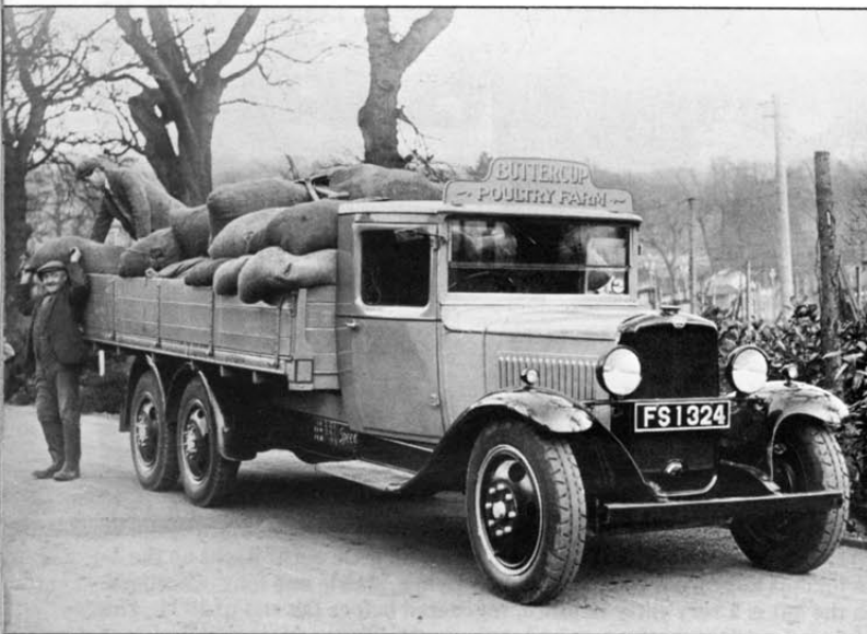
Six-wheeler conversions (above) and articulated outfits appeared during Bedford's very first year. Both Baico and Spurling soon offered chassis extensions and third axles. Oddly, the very early 2-tonner at left above sported single rear wheels, unlike the more usual twin
