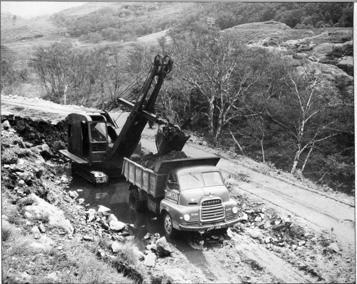
Above, the 1957 new-look radiator grille on an S-type 7-ton tipper and (right) on a C-type 5-tonner. The 4-, 5- and 6-ton C models shared the looks of the S-type 'Big Bedfords'. Lower picture is of a 12-seater Spurling crew car on a D-type 25 cwt chassis.
