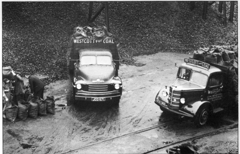
models in 1953. Known as the Middleweights, they introduced the first-ever diesel engine option in Bedfords, the Perkins P6V. Note the contest (below) between the A models and their predecessors.
