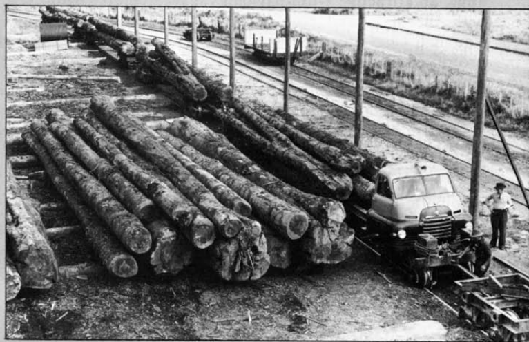
was mounted on a rail bogie, its engine had three carburetors and it spent many years hauling 50-ton loads of timber in a New Zealand lumber siding with 1 in 10 gradients.
