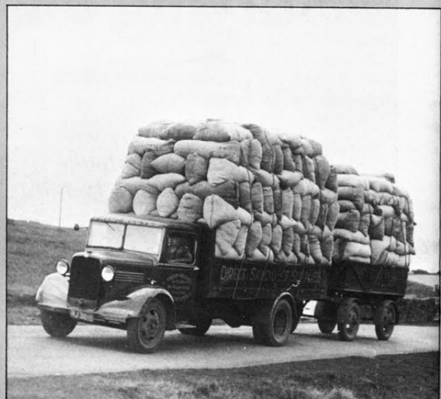
problems while the sawdust-carrying 3-tonner at right looks more than 50% overloaded even without the drawbar trailer. Today's much more rigid regulations do at least prevent such hazards.
