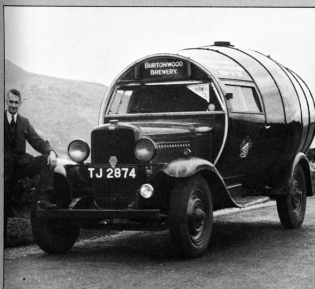
BODIES UNBEAUTIFUL: Beneath that ugly barrel body on the left is a WS 30 cwt chassis of the earliest type – certainly pre-1935. Eyecatching certainly – which was the idea. The 10-seater vehicle at
