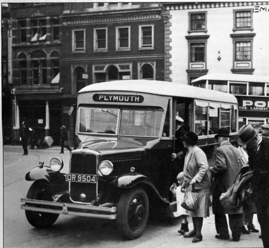
In August 1931 came modified versions of the 2-ton chassis for bus bodywork, the WHB for 14-seater bodies, the WLB for 20-seaters. The Waveney-bodied 14-seater (above) was the very first bus to be built on this chassis; it has now been faithfully restored by Bedford dealers Arlington Motors. The Plymouth owner of the Duple-bodied 20-seater (below) called the Bedford "far and away the best 20-seater on the market".
