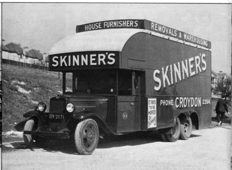
wheels on both rear axles. Modified 2-ton chassis for semi-trailer operation, like the two shown below, were offered by Carrimore and Scammell during Bedford's first year. The first purpose-built Bedford tractor unit did not appear until 1939.
