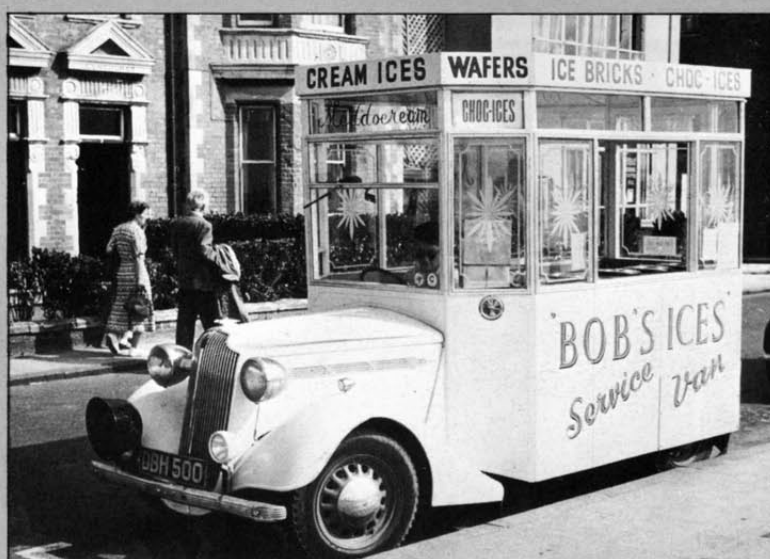
a mild piece of editorial licence – the basis of the 'glasshouse' ice-cream van is a 1936 DX Vauxhall saloon, which before its transformation worked for a number of years as a taxi.
