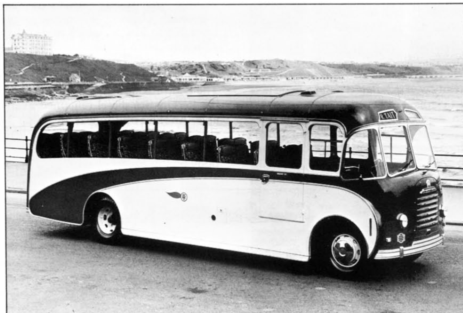
Pictures here represent the four original S-type 7-tonners. Facing page, the short-wheelbase tipper version; top here, the 10-ton tractor unit; centre, the 156 in.-wheelbase rigid for a full 7-ton payload; lower, the 206 in.-wheelbase SB bus/coach chassis, this one with Plaxton body. The S models were Bedford's first civilian trucks with the full forward-control treatment.
