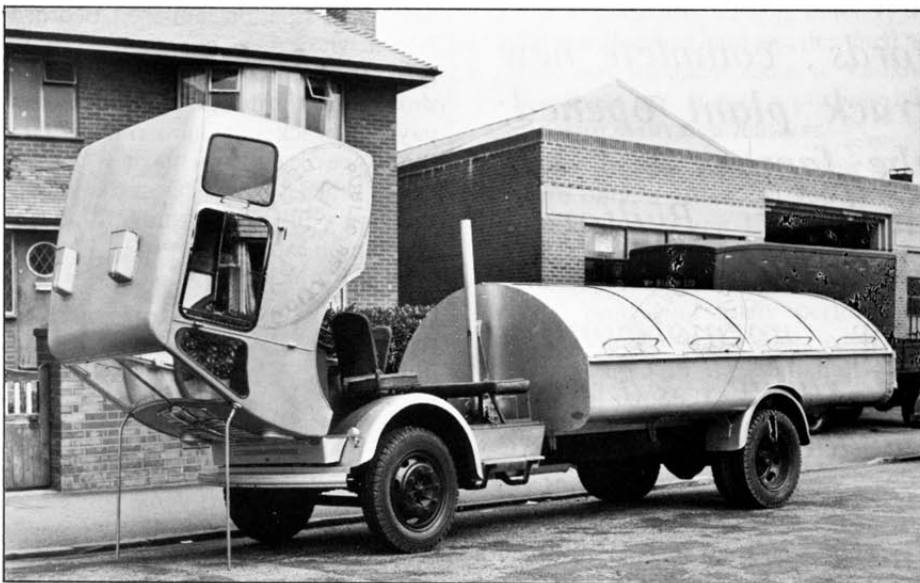
Interesting body styles on the K, M and O Bedfords. The flat-fronted roundsman's delivery vans (top) are on the K 30 cwt chassis. The smartly liveried job in the centre, on a 5-ton chassis, has a bonnet-less, full-tilt cab conversion designed by Nevilles. Note the long hinges just below each headlamp. The Eagle 10 cu yd refuse collector, lower picture, also on a 5-ton long chassis, shows how the Neville tilt cab gave really clear access to the engine and the whole of the large crew-cab.
